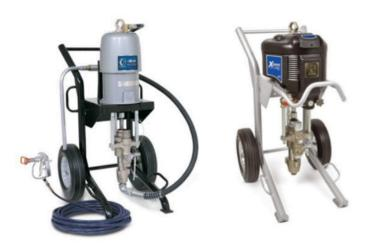
Minimum Requirements: 33:1, 100CFM, 120psi constant, 3/4" to 1.25" air delivery line. Air hose feed must be a minimum 3/4"delivery to the unit. 3/8" air hose is not large enough to power the above units efficiently.
