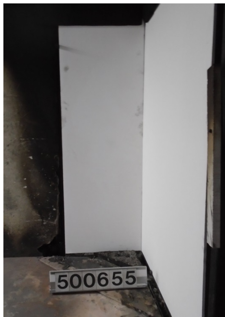
Plate 2: Close up view of the vertical outer edge of the long wing at a height of 500mm
