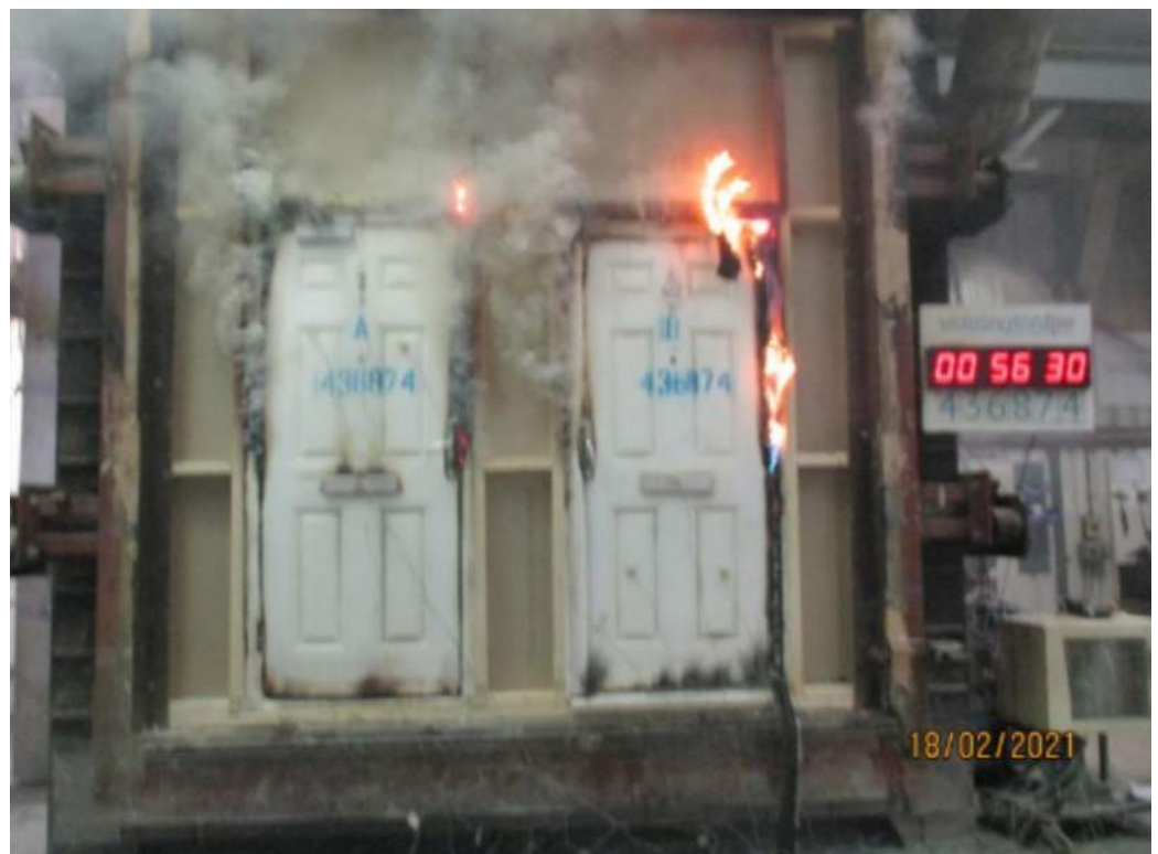
The unexposed face of the doorsets after a test duration of 56 minutes
