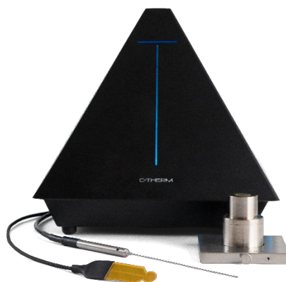
Figure A5. C-Therm's Trident Controller with all 3 sensor types (MTPS, TPS and TLS)
