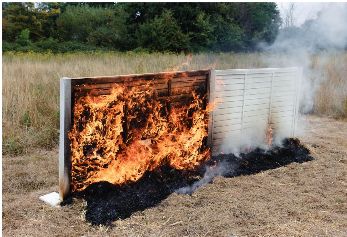
Figure 2 Testing Zenova Fire resistant paint
